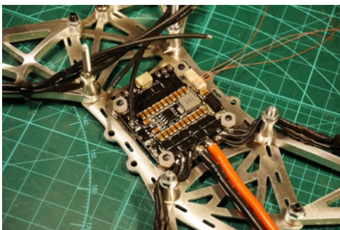
Sample of phase cables soldered to a DYS 4in1.
